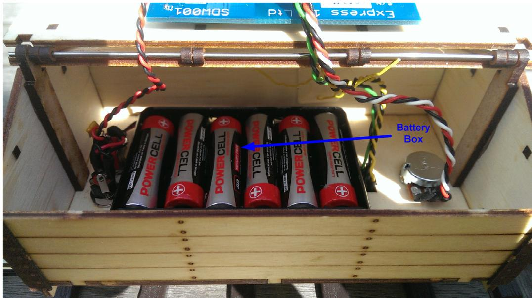
The battery box accommodates 6 off AA batteries and is located on the inside of the base of the wagon. Any batteries supplied are non-rechargeable so that the wagon is 'ready to run': the owner can then choose his/her preference of rechargeable batteries.
