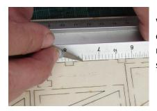
1) Cut the parts from the frets with a sharp modelling knife. We find it best to place the frets face down on a cutting mat and cut through the short "bridges" with the aid of a steel rule. Do not be tempted to simply twist the parts out the fret, this may splinter some of the edges.
