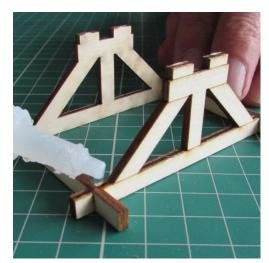
8) Assemble the stand by dropping the half notched cross pieces over the stand frame pieces (checking the engraved joint lines are facing outwards) and fix with a few drops of super glue.
