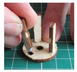
3 ) Place a drum side "planked face" down on your modelling mat and insert one end of each of the 18 drum segments into the ring of holes. The segments are deliberately slightly loose in their holes. (Don't be tempted to glue them at this point).
