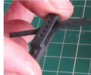
Thread the steel rod through the holes of the 2 "V" hangers and glue the top of the ratchet into a locating hole in the sole bar. Secure the brake arm in place with a couple of drops of glue where the rod passes through the "V" hangers.
