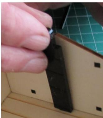
Now glue the internal end hinge plates in place. Each has a “foot” which should locate in a hole in the wagon floor to help you position the part correctly.
