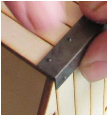
Once the body glue is dry; glue the corner plates on to the four corners. Be careful to align the top of the plate with the top edge, if it is too high it will prevent the lid from closing properly.
