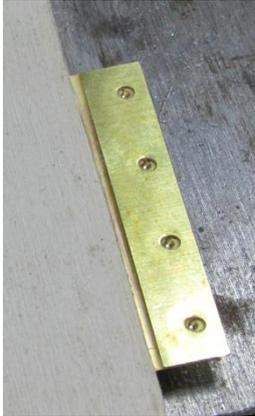
Find two pieces of scrap plywood (e.g. from the body fret) and place a corner plate along one edge with its “fold line” aligned with the plywood’s edge.
