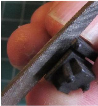
The internal surfaces of the horn block may still have traces of “printing” powder on them that will need cleaning off. With a small flat needle file, lightly file the 3 internal faces (that slide into the horn guide) to remove any of this residue.
