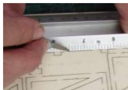
DO NOT simply try and twist the parts out of the fret, there is a risk that the part may tear. The laser cutting process will leave a degree of edge discolouration. If you plan to leave your model unpainted now is the time to lightly sand the edges to remove this discolouration.
