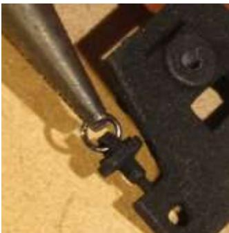
First poke a pin or thin drill bit through the hole to clear any printing powder.
