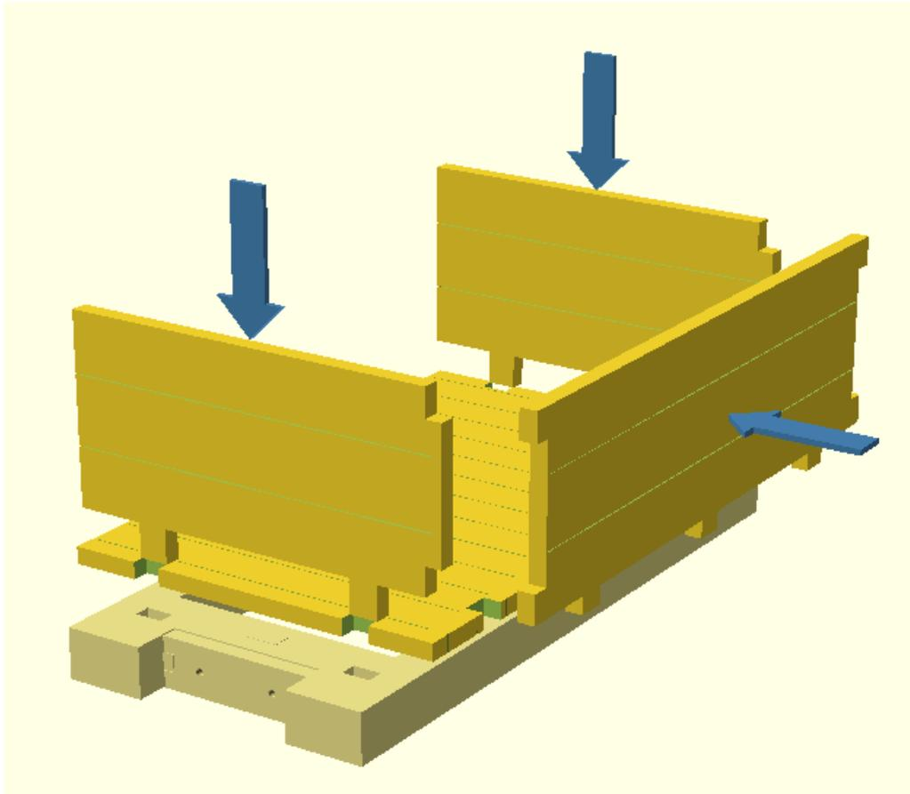
Glue one body end and the body side to the floor. Now glue the other end onto the assembly. Finally glue the body onto the chassis. The locating pegs on the body ends should locate in the sockets in the chassis.
