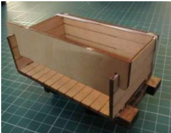
Lightly clamp or slip on a rubber band or two. The kit includes a temporary jig to slip over the body ends as shown in the photo, to stop the ends bowing in whilst the glue is setting.
