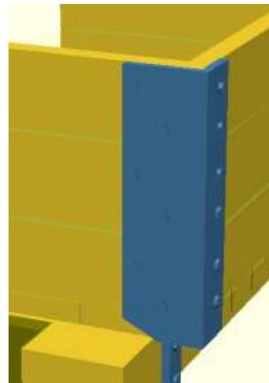
On the other side of the wagon glue the corners plates. Note the chamfer is at the bottom just above the dumb buffer.
