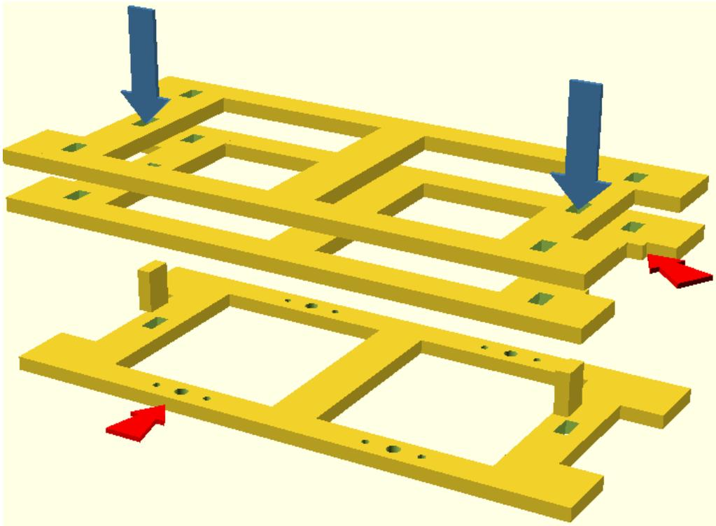
PVA wood glue is recommended for these steps or if you want to use a super-glue DON'T use an "instant grab type". Glue the 3 "chassis plates" together using the small rectangular locating pegs at each end. Note the sequence of axle box holes; small tab on "buffer"; and no tab of the three plates. Make sure the parts are squeezed together properly. Wipe out any glue that oozes into the body end locating holes.
