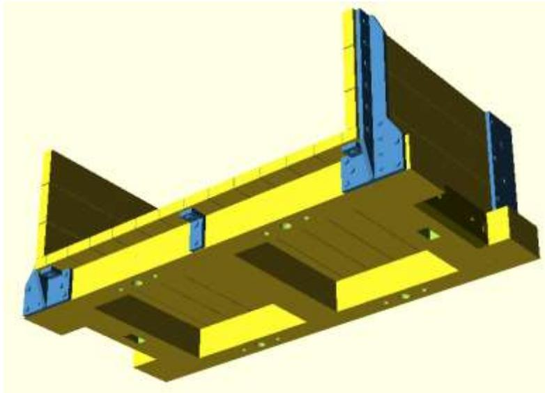
Glue the two “edge supports” either side of the opening as shown. A good quality super glue works well for this.
