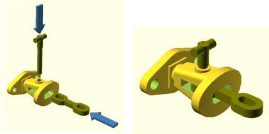
The modeller has the choice of using this coupling in a prototypical manner; i.e. keeping the link engaged in one buffer and sliding the t-pin in and out of the other ( tweezers recommended) to couple the wagons together.
