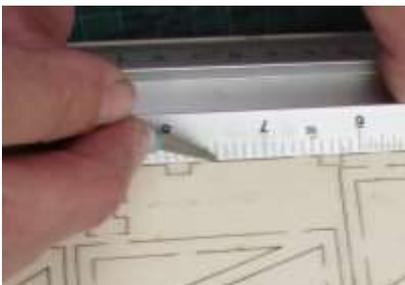
DO NOT simply try and twist the parts out of the fret, there is a risk that the part may tear. The laser cutting process will leave a degree of edge discolouration. If you plan to leave you model unpainted now is the time to lightly sand the edges to remove this discolouration.
