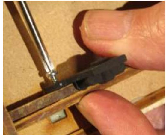
Fit the opposite axle guard to a wheel journal and then thread the opposite journal into the "semi-fixed" axle guard. Now gently manoeuvre the unfixed axle guard into position. Fasten in position with two more screws (do make sure they go into their pilot holes). Tighten up the screws on the first axle guard.
