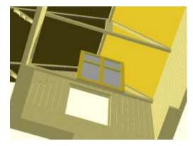
10) Glue the 4 window assemblies into their recesses from the inside of the building aging using thin beads of contact adhesive. Note that the white window frame is on the outside of the clear glazing.
