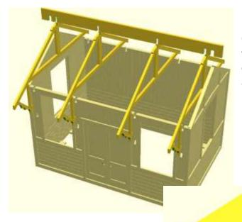
6) Glue the 4 rafters into their sockets in the wall tops. (These sockets may need cleaning out with a file first if the overlays aren't aligned perfectly). Then glue the roof ridge beam in place. Allow glue to dry.
