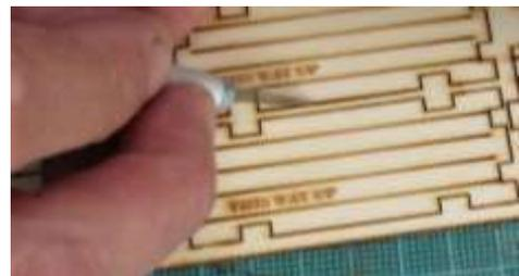
Most parts are attached to their frets by small sections of half cuts. To remove parts either cut through the remaining material from the front with a thin sharp blade (e.g. a scalpel) on a cutting mat or turn the whole fret over and with the aid of a steel ruler aligned with the pieces side, cut lightly with a knife to break through the remaining wood.
