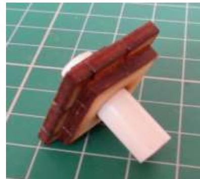
7) Now is a good time to paint the chimney. A quick way is to spray it with red oxide car paint primer from a “rattle can”.
