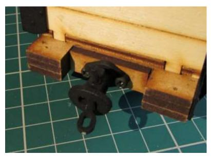
Either way, fix the two couplers onto the wagon ends with four self-tapping screws. Again it is suggested you chemically blacken these or use some matt black enamel paint on the screw heads.
