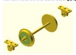
It is suggested that you chemically blacken (e.g. Carr's Metal Black) the 8 screws that fix the axle boxes in place. If not, you can always but a touch of matt black enamel paint on the screw heads later on.
