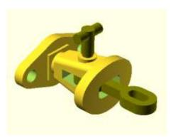
The modeller has the choice of using this coupling in a prototypical manner; i.e. keeping the link engaged in one buffer and sliding the t-pin in and out of the other ( tweezers recommended) to couple the wagons together.
