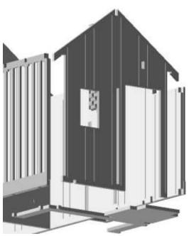
Next glue the door end wall in place together with the end brace (which includes the porch floor and doorstep).
