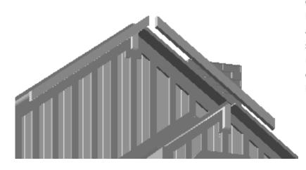
Cut the four parallelogram barge board spacers from the 3mm frets and glue onto the gable ends; either side of the roof ridge beam, tucked up right under the roof panels. They are designed to give a surface to glue the barge boards onto (next step).
