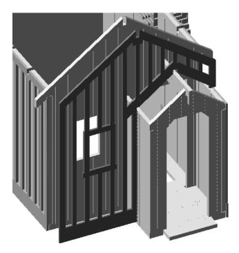
Next glue the planking overlays onto the porch
