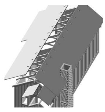
Before gluing the main roof panels in place; use them as templates to cut the plastic "slate" overlays to shape. Trick is to align the bottom edges of the panels to a horizontal slate course so that you get a complete tile at the bottom. The top edge will be covered by the ridge piece so a partial tile course does not show.
