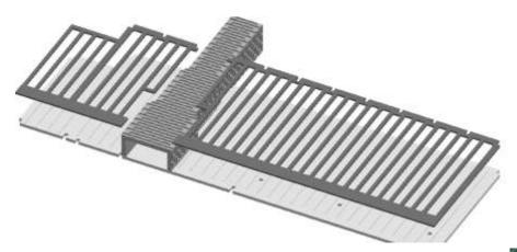
Glue the back overlays (1.5 mm ply) onto the back wall (3 mm ply). The top and bottom edges should be flush and the side edges should overlay the locating lugs on the wall sides. Clean off any glue that oozes onto the front face or onto the side edges. Place something flat and heavy on top of the two overlays and wait for the glue to set
