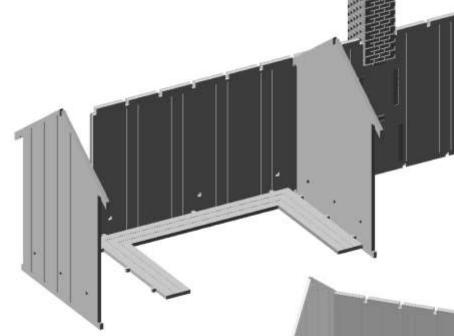
Glue the plain centre wall and waiting room seat to the back wall. (You may find you have to ease the two sockets in the back wall with a small file). Next glue the planked end wall (planks outward) to the assembly.
