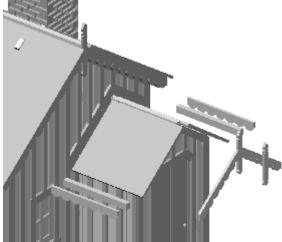
Cut the two small porch valancing supports from their 3mm frets and glue them to the top of the porch walls right under the porch eaves. Next glue the porch valancing strips to them and finally the porch barge boards to the porch gable end.
