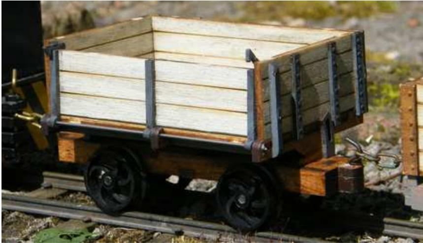
Side tipping or dumping wagons were extensively used by narrow gauge industrial railways and range in size from small hand propelled examples up to large wagons capable of carrying several tonnes hauled in long rakes by large locomotives (e.g. the Kettering furnaces railway).
