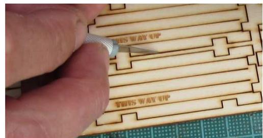
**DO NOT** simply try and twist the parts out of the fret, there is a risk that the part may tear. The laser cutting process will leave a degree of edge discolouration. If you plan to leave you model unpainted now is the time to lightly sand the edges to remove this discolouration.
