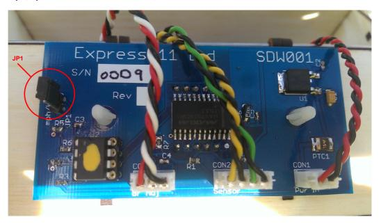
JP1 is located on the controller printed circuit board (pcb) that is mounted on the inside of the one of the 'flip over' covers of the wagon.
