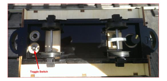
The wagon is OFF when the switch is in the centre position
