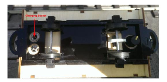
The 2.1mm positive inner pin charging socket is present so that, if rechargeable batteries are fitted, these can be recharged in situ using a proprietary 'smart' charger.
