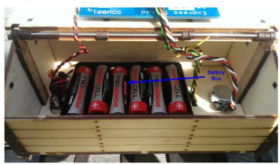
The battery box accommodates 6 off AA batteries and is located on the inside of the base of the wagon. Any batteries supplied are non-rechargeable so that the wagon is 'ready to run': the owner can then choose his/her preference of rechargeable batteries.
