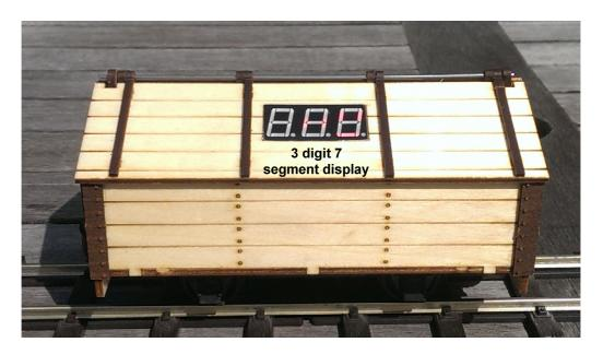
The display indicates the scale speed in miles per hour (mph) or kilometers per hour (kph), depending on the absence or presence respectively of the shorting header across pins 1 and 2 of JP1 on the controller circuit board (item 2).
