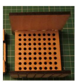
2) Glue the lower spacing plate (the one with the drainage holes and locating lugs) between the front and back pieces.
