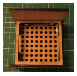
4) Glue the stepped side pieces in place. Hold the complete assembly together with a rubber band. With a damp cloth wipe of any excess glue that has oozed out of the joints on the outside of the buffers. Allow the glue to dry before taking the rubber band off.
