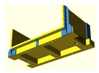
Glue the two "edge supports" either side of the opening as shown. A good quality super glue works well for this.
