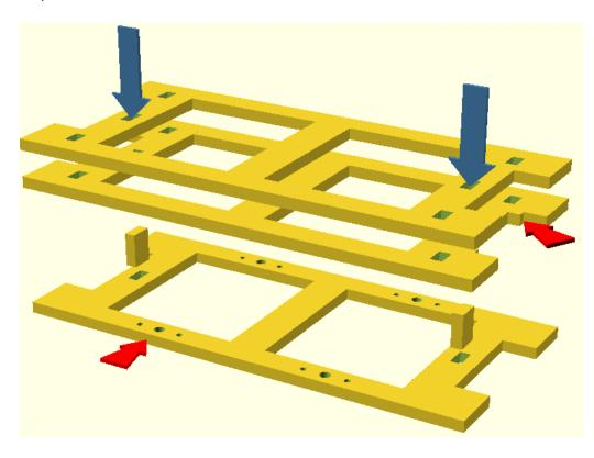
PVA wood glue is recommended for these steps or if you want to use a super-glue DON'T use an "instant grab type". Glue the 3 "chassis plates" together using the small rectangular locating pegs at each end. Note the sequence of axle box holes; small tab on "buffer"; and no tab of the three plates. Make sure the parts are squeezed together properly. Wipe out any glue that oozes into the body end locating holes.
