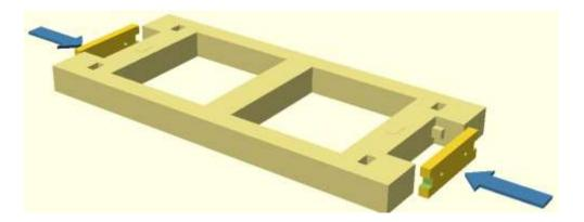
Now glue the two buffer mounting plates onto the ends between the two dumb buffers.
