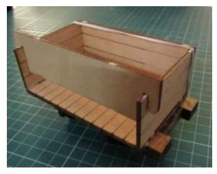
Lightly clamp or slip on a rubber band or two. The kit includes a temporary jig to slip over the body ends as shown in the photo, to stop the ends bowing in whilst the glue is setting.
