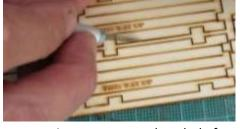
material from the front with a thin sharp blade (e.g. a scalpel) on a cutting mat or turn the whole fret over and with the aid of a steel ruler aligned with the pieces side, cut lightly with a knife to break through the remaining wood.
