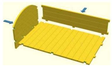
Step 4 Now glue an end and side to the plywood floor
