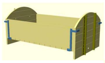
Step 9 Glue the four corner hinge assemblies onto the corners as shown.
