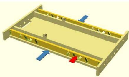
Step 3 Glue the 2 plywood outer sole bars on the outer faces of the MDF solebars.
