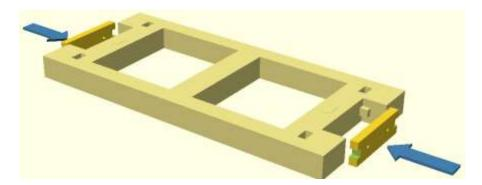
Now glue the two buffer mounting plates of your choice (see below) onto the ends between the two dumb buffers. Once the glue has set, lightly sand the edges of the "plates" that now form the sole bars and dumb buffers to remove any excess glue and to provide a good surface to paint or varnish.
