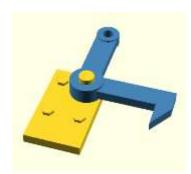
Push, but do not glue, the door latches onto their mounting plates. Note there are left and right handed mounting plates. Make sure that the back of the parts are sprue free and flat. You will probably have to clear printing powder from the hole with a small drill bit or piece of wire.
