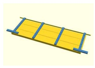
Now thread the hinge rod through the hinge eyes (but don't glue them) and place the hinge plates on the door as shown. One side of the door has engraved lines to help you align the plates evenly.
