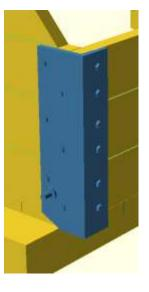
Glue three floor support angles onto the sole bar as shown.
