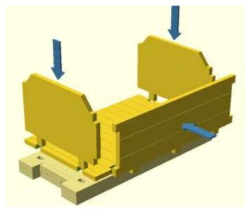
Glue one body end and the body side to the floor. Now glue the other end onto the assembly. Finally glue the body onto the chassis. The locating pegs on the body ends should locate in the sockets in the chassis.
