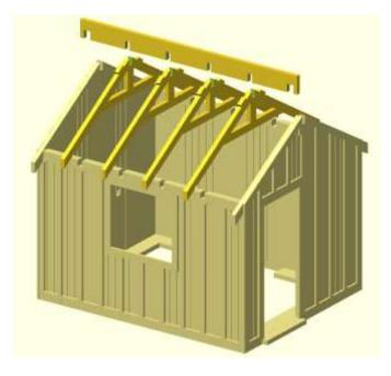
10) Glue the 4 rafters into their sockets in the wall tops. (These sockets may need cleaning out with a file first if the overlays aren't aligned perfectly). Then glue the roof ridge beam in place. Allow glue to dry.
