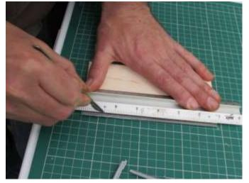
12) Once set, trim off the excess overlay from behind using a ruler and sharp knife.
