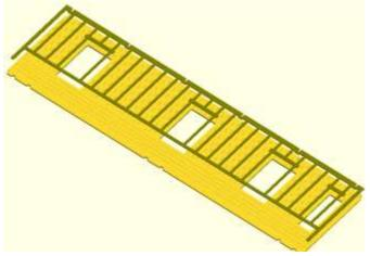
Glue the back overlay (1.5 mm ply) onto the back wall (3 mm ply). The top and bottom edges should be flush and the side edges should overlay the locating lugs on the wall sides. Clean off any glue that oozes onto the front face or onto the side edges. Place something flat and heavy on top of the assembly and wait for the glue to set
