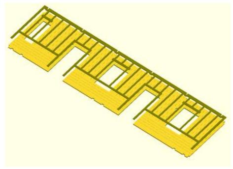
Glue the top overlay (1.5 mm ply) onto the front wall (3 mm ply) and the door assembly into its recess. The edges should be flush like the back wall. Again clean off any excess glue (particularly in the window frame recesses) and set aside to dry.
