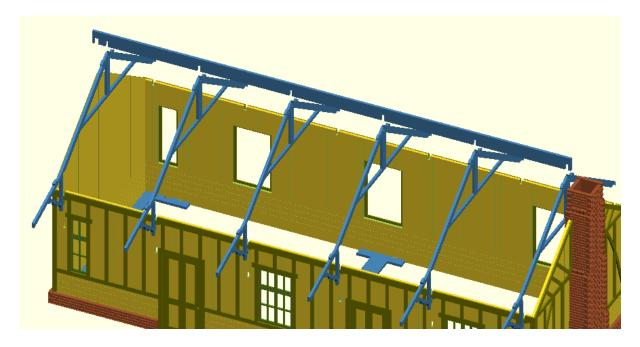
Glue the 6 rafters into their sockets in the wall tops. (These sockets may need cleaning out with a file
