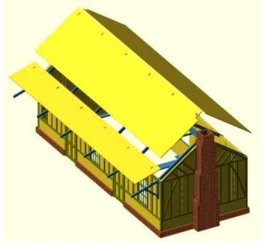
Now glue the roof overlay onto the roof. Our preferred method is to coat the underside of the overlay with the glue. Line up the fold with the ridge beam and first rub *down* the front roof overlay making sure you don't get it "skewed".(Imagine you are hanging wallpaper). Then rub down the back overlay. This way you shouldn't get any bubbles under the overlay. Finally use 2 scrap pieces of wood and some clamps to hold in place while the glue sets.
