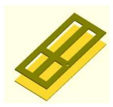
Glue the door overlays (1.5mm ply) onto the door backs (1.5 mm ply) making sure all edges are flush. Again place under a flat weight and allow glue to set. Again it may be advisable to prepaint these parts now.
