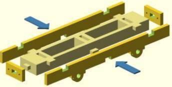
Glue the two sole bars onto the sides and then the two end plates.
