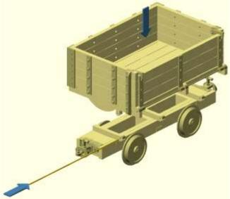
You can either use the "T pin" and link to couple the wagon or simply loop the supplied 3 link chain of the "T pin" and use as a standard centre buffer.
