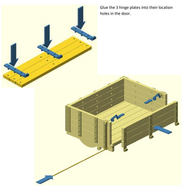
Locate the door hinges between the hinge holes on the chassis. Slide the long steel rod through all 6 holes. Fix in place with 2 small drops of super glue on the outer ends of the rod.
