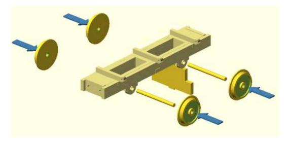
Push one wheel onto an axle, pass the axle through a bearing tube in the chassis and fit another wheel to the other end. Gently squeeze the two wheels together in smooth jawed vice until the
