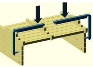
Glue the 7 strapping strips into their locating holes in the body side and end.
