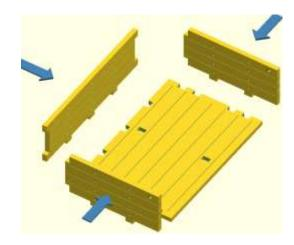
Glue the 3 floor cross pieces onto the floor bottom.
