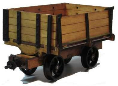
Side tipping or dumping wagons were extensively used by narrow gauge industrial railways and range in size from small hand propelled examples up to large wagons capable of carrying several tonnes hauled in long rakes by large locomotives (e.g. the Kettering furnaces railway).
