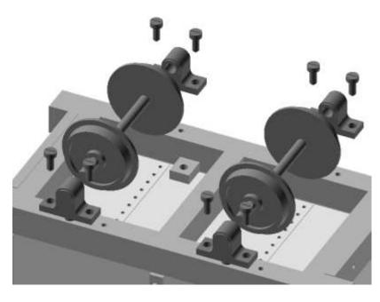
Place a pair of axle boxes onto an wheel set and fit the two locating pegs into their holes in the chassis. Now secure in place with 4 of the self tapping screws.
