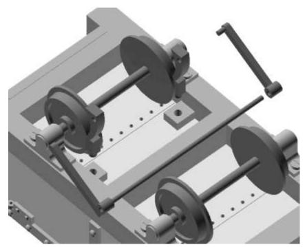
Fit the 2 brake arms onto the 1.5 mm diameter rod and then clip the arms into the outside of the brake shoes, but don't glue anything yet.
