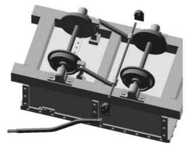
Included in the kit is a short length of fine chain. Gently open one of the small links and thread it through the bracket on the top strapping and then close the link. Thread the brake handle
