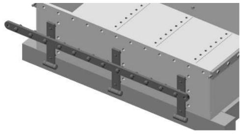
On the door side glue the top strap in place, the end lugs should locate over the pins on the end strapping.
