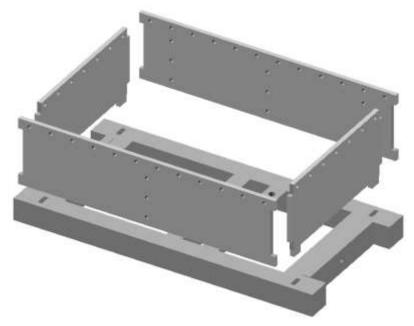
Separate the 4 body sides from their frets with a sharp knife. Peel off the backing film before gluing them together,
