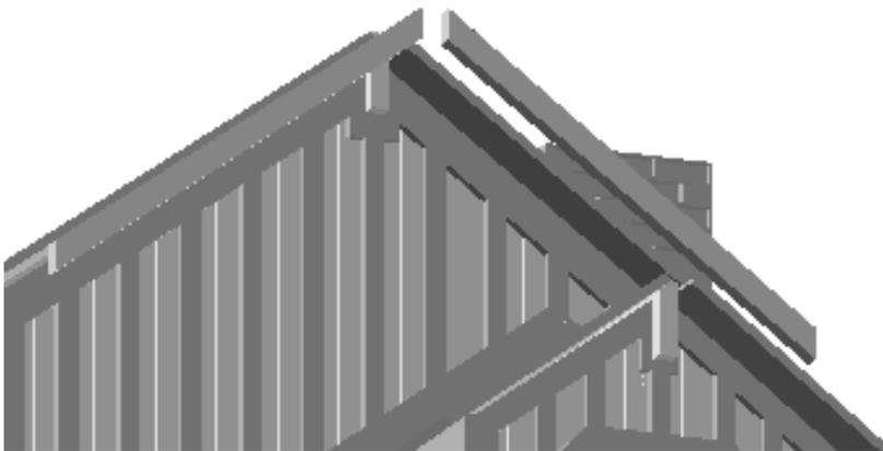
Cut the four parallelogram barge board spacers from the 3mm frets and glue onto the gable ends; either side of the roof ridge beam, tucked up right under the roof panels. They are designed to give a surface to glue the barge boards onto (next step).
