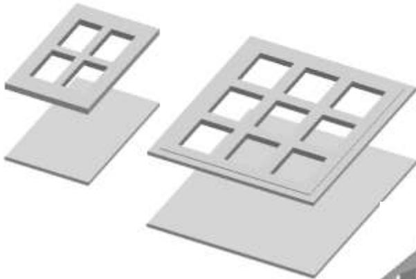
Cut the two window frames from the 1.5mm “fret” and paint them. Glue the wooden window frames to the clear plastic glazing.
