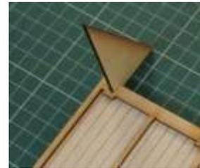
TIP: Temporarily push a couple of scraps of 3 mm ply into the slots to help align the parts.
