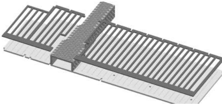
Glue the back overlays (1.5 mm ply) onto the back wall (3 mm ply). The top and bottom edges should be flush and the side edges should overlay the locating lugs on the wall sides. Clean off any glue that oozes onto the front face or onto the side edges. Place something flat and heavy on top of the two overlays and wait for the glue to set
