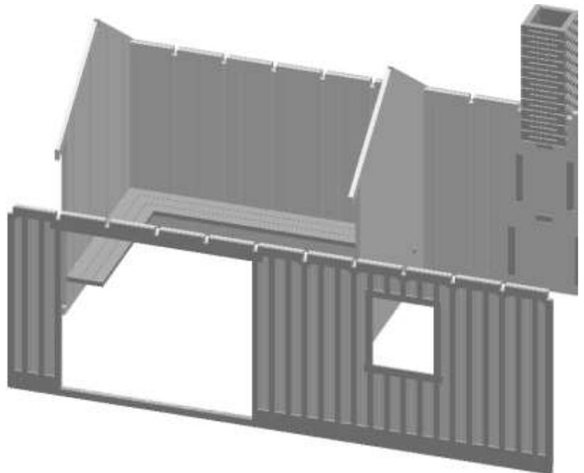
Next glue the door end wall in place together with the end brace (which includes the porch floor and doorstep).
