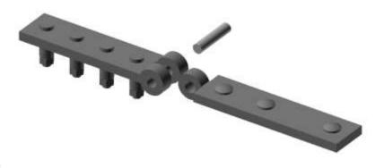
Push the rod into the hinges as shown. (You shouldn't need any glue)
