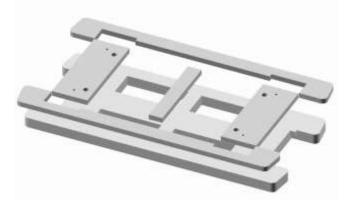
Sand any roughness off the two pairs of 3D printed mounting beams. Ensure they fit together nicely before gluing the chassis beams to the chassis. Note that the tapered lugs face outwards on the chassis.
