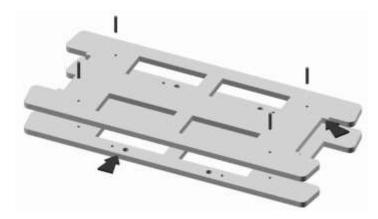
PVA wood glue is recommended for these steps or if you want to use a super-glue DON'T use an "instant grab type". Glue the 2 "chassis plates" together using four 9mm lengths cut from the supplied 1.5 mm diameter brass rod in the locating holes at each end.
