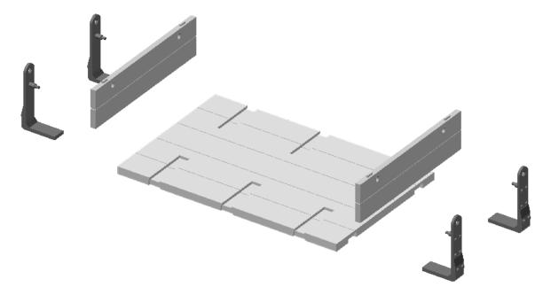
Glue brackets to the wagon ends (pushing the door hook pivots through the locating holes in the wagon ends and then glue the ends/brackets to the wagon floor.
