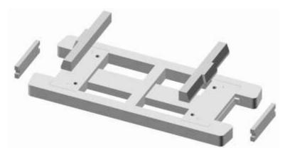
Now glue the two buffer mounting plates onto the ends between the two dumb buffers. Once the glue has set, lightly sand the edges of the "plates" that now form the sole bars and dumb buffers to remove any excess glue and to provide a good surface to paint or varnish.
