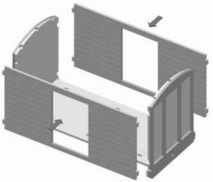
Step 6 Glue the two side overlays in place.
