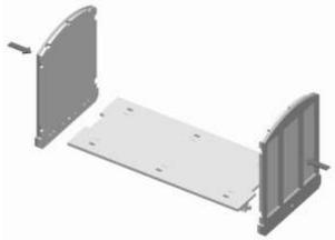
Step 4 Now glue ends onto underframe from step 2.
