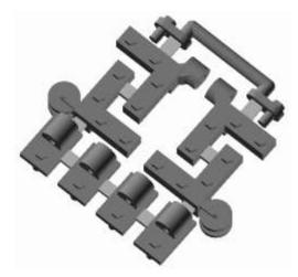
Prepare the door detail components by removing the "sprues" (the light sections in the picture) that hold the parts together with a sharp modelling knife or miniature side cutters. If necessary clean any printing dust off the "castings" with a toothbrush. "Twizzle" a 1.5 mm drill bit in the holes in the top door runners so that they slide on the supplied door rods.
