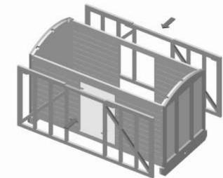
Step 7 Glue the floor overlay (1.5 mm ply) onto the MDF floor.
