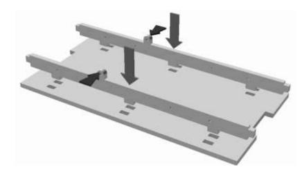
Glue the 2 MDF inner sole-bars into the locating sockets of the MDF under floor. The inner hole sets are for 32mm gauge and the outer set for 45nmm gauge. Make sure that the brake hangers are opposite each other as indicated. Make sure the parts are squeezed together properly. Wipe off any glue that oozes out of the joints.
