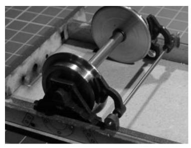
Thread a brake rod (two are provided to cater for either 45mm or 32mm gauge); through a brake hanger; through the two shoes and out through the other brake hanger. The rod should be almost flush on the side where the brake ratchet's locating hole is at the "brake end" (see photo) and should protrude 6mm about the other side.
