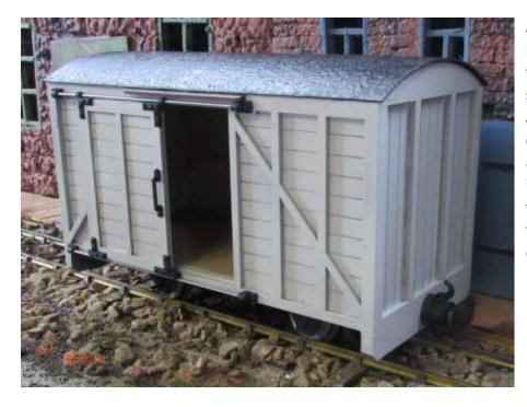
A pair of Binnie centrebuffer is include with this kit but correctly spaced pilot holes for Accucraft chopper couplings (not included) are provided in the inner buffer beams so that the modeller may fit these buffers if desired.
