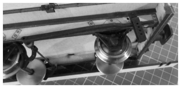
TIP A lever retaining pin can easily be made from a bent paper staple.
