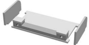
Trap two M2 nuts in the front cab foot with four of the long plastic tabs (again temporarily fitting two M2 screws in place helps). Then glue the brake quadrant to the right hand side of the cab foot.
