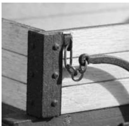
Included in the kit is a short length of fine chain. Cut either 2 or 4 links from this and push one end link through the split ring at the end of the brake handle and then seal with a spot of glue and dab of paint.
