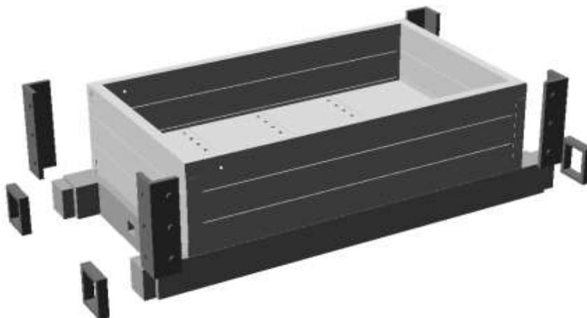
Glue the corner plates and buffer straps (if required) in place.
