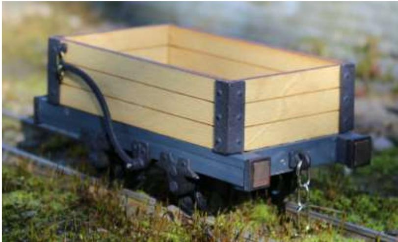
A choice of couplings is included in this kit. You can either assemble the wagon with side "dumb buffers" and a central hook for a 3 link chain (see above) or if you prefer a centre buffer (for greater compatibility with the rest of your stock) , a pair of Penrhyn style wagon buffers are also included (see below).
