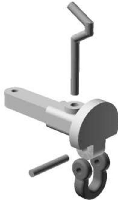
Now push the hook or buffer shank through the rectangular socket in the buffer beam and push a small (6mm) section of brass rod through the hole to fix in place.
