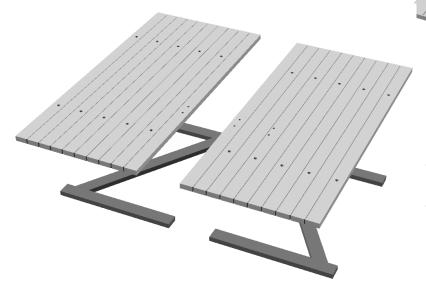
Now glue the "Z" frames to the back of the main shed doors (both 3mm thick). Take care with the positioning of the door catch locating holes which are towards the bottom of the doors. Ensure no glue oozes into the door hinge strap locating holes.
