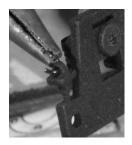
Fit the axle guards to the wheels and then screw the axle guards to the inner sole bars. Note pilot holes are provided on the inside of the sole bars to aid in accurate location of the axle guards
