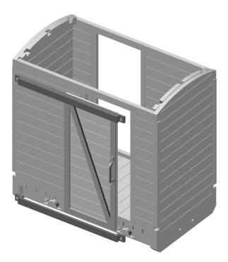
Glue the top and bottom door runners in place above and below the door openings, trapping the doors in place. Ensure no glue gets on the door edges.
