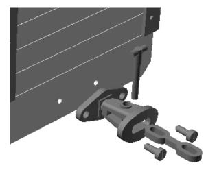
Screw the bell mouth couplers in place with 4 self-tapping screws
