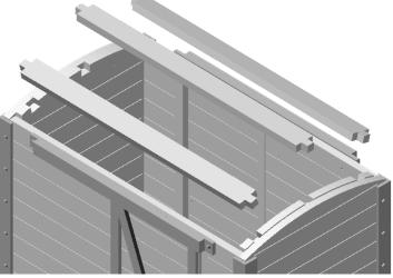
Glue the three roof supports in place and allow glue to set
