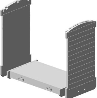
Glue the two body ends to the chassis ensuring the bottom edges are flush.
