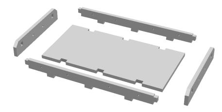
Glue the 2 MDF inner sole-bars and 2 MDF buffer beams to the MDF floor. The parts should fit together snugly but if necessary lightly file the lug edges if the fit is too tight. Make sure the parts are squeezed together properly. Wipe out any glue that oozes out of the joints
