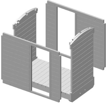
Glue a body sides to the floor and end wall. Note that the section above the door opening is wider than the section below the door opening.
