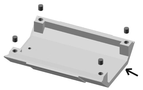
Clean out the four holes with a 3mm drill bit and then glue a magnet into each hole.
