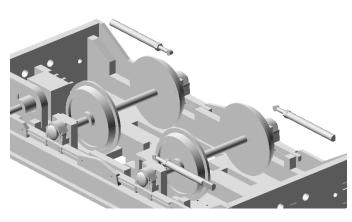
Glue three "thrust rods" into place between axle boxes and the frames ends (see below)
