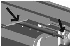
The round ends locate in a little socket in the axle box side and there is a little flat to glue onto the frame.
