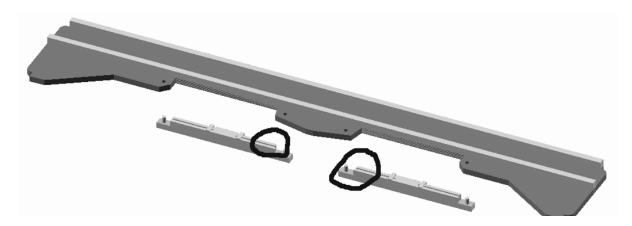
Glue two of the springs into their locating holes in the outer frame plates. Note these parts are "handed" and the sloped cut outs go in the centre. The flat surface of the spring is at the bottom and the slightly raised "clips" are at the top. Repeat for other side.
