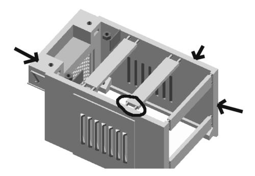
Next carefully remove the bottom rectangular printing supports by snipping the joining cylinders (circled) with side cutters .
