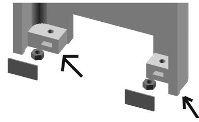
Clean out the two bolt holes in the "nut cages"
