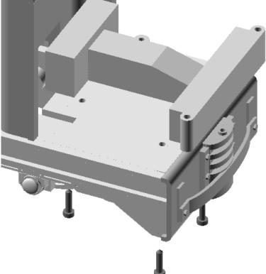
Fix the rear sandbox/transmission tunnel to the back of the footplate with three self tapping screws.
