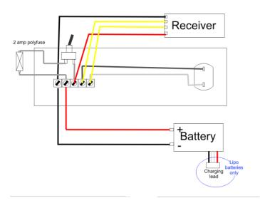
However if you fancy fitting radio control there is sufficient room in the bonnet cavity to accommodate either a 3 cell lipo battery and a Deltang RX60 or a 4 cell AAA Nimh battery pack and a Locoremote Mini B (pre wired leads recommended). In the latter case we would recommend one of the 6 volt motors.
