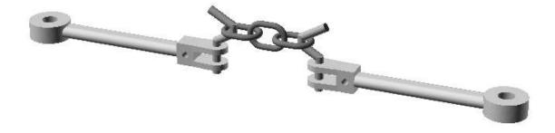
Thread the drawbars through the slots in the body above the buffers and place the pivot bosses over the pivot bolts. You may have to widen the pivot hole with a 3mm drill bit to do this.
