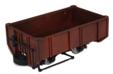
This model is based on the steel open wagons built at Tindharia works on the Darjeeling Himalayan Railway in India. Their design was largely based on the Leeds Forge wagons imported in the early 1900s but were fabricated from steel section and plate rather the originals drop forging.
