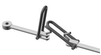
the nail point off. Bend up a pair of simple wire hooks and glue into the vertical holes at the end of the both drawbars.
