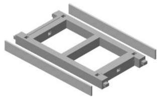
If you are intending to use our hook and chain couplers, glue the 4 small sole bar extensions onto their locating lugs (the 3D printed buffer straps will glue around these later).
