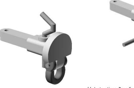
Now push the hook or buffer shank though the rectangular socket in the buffer beam and push a small (6mm) section of brass rod though the hole to fix in place.
