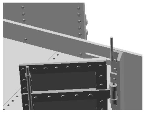
Cut eight 12 mm lengths of brass wire. Attach the doors to the door frames by carefully inserting the brass pivot wires through the 3 holes. If necessary secure with a drop of super glue to an outer end of the pivot wires
