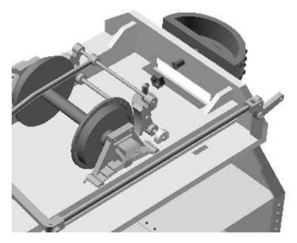
Thread a M3 hex head bolt into each of the buffers. Place the body onto the chassis and secure by pushing the M3 bolt through the central holes and securing behind with a M3 nut.
