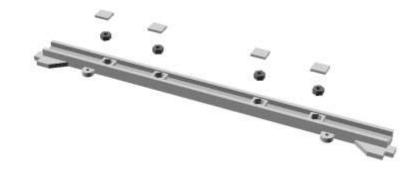
Glue four small "nut cover plate" in place to trap the nuts. "Twizzle" a 1.5mm drill bit in the brake hanger holes so that the steel brake shoe rods fit.
