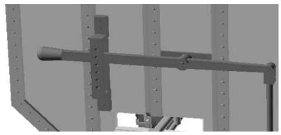
Glue the hand rail at the top of the brake end. N.B. you may find it easier to trim off a couple of rivet heads on the "angle iron" so that you get a flat surface to glue to.
