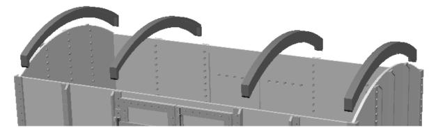
Glue the four roof supports in place. The sides of the end supports should be glued to the body ends to give a nice firm joint.
