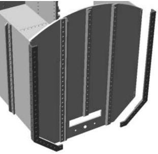
Clean the door hinges out with a very small drill bit or fine reamer. Glue the door straps to the doors with super glue or epoxy.
