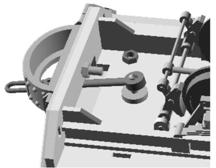
Thread the drawbars through the slots in the body above the buffers and place the pivot bosses over the pivot bolts. You may have to widen the pivot hole with a 3mm drill bit to do this.
