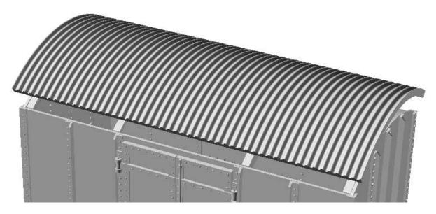
Trim the vacuum formed roof sheet to size and glue to the four roof supports with something like epoxy resin.
