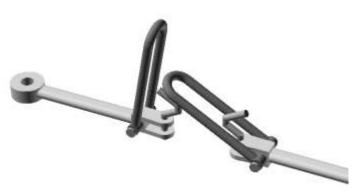
outsides. Bend up a pair of simple wire hooks and glue into the vertical holes at the end of the both drawbars.
