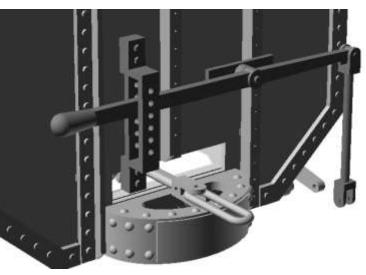
N.B. the ratchet plate should be on the body end hard up against the angle iron.
