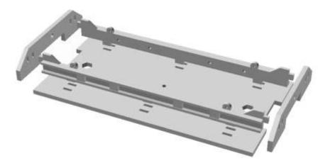
Glue the two sole-bars into the locating sockets of the MDF under floor. The inner sockets are for 32mm gauge and the outer set for 45mm gauge. Glue the two MDF buffer beams onto the sole bar lugs.
