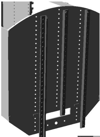
Glue the end straps in place. Note there are left and right hand end straps. Glue a shorter side strap in the middle. **Again note the orientation of the straps which is important for fitting the brake lever later.**
