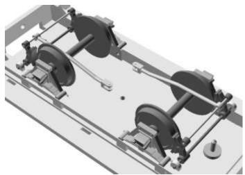
Slide one of the steel brake rods through a brake hanger hole, through the larger bosses of a pair brake shoes and finally through the opposite brake hanger. Adjust the brake shoes so they are in line with the wheel treads but outside of the rims. Tread a length of brass rod through the other shoe bosses and the link arm boss and trim to length. **N.B. the link arm is slightly cranked and the central end is closer to the floor**
