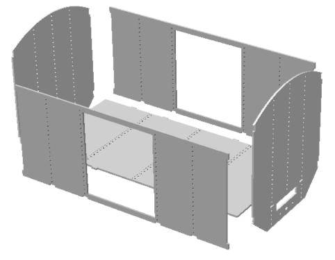
Glue the sides and ends to the body floor. Liquid styrene cement (e.g. MEK) works well here but super glue will do. Make sure the rivet detail on the floor faces upward!
