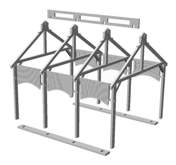
Glue the six side panels into their locating sockets in the four main "A frames" and the bottom of the "A frames" into the two base strips. This will help to keep the four frames in-line
