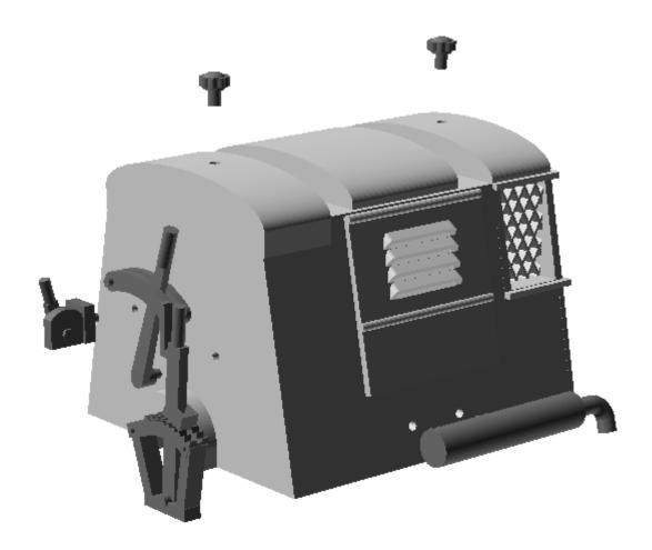
Glue the filler caps, control levers and exhaust silencer to the bonnet. A good quality super glue or aero modellers canopy glue may be best for this step if you have already painted the bodywork as "plastic weld" will take the paint off!
