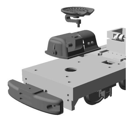
Temporarily fit the seat into it locating hole in the gear box top, you will probably need to ream out the hole slightly. Remove the seat for now, we will glue in place later.
