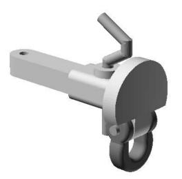
Now push the hook or buffer shank though the rectangular socket in the buffer beam and push a small (6mm) section of brass rod though the hole to fix in place.
