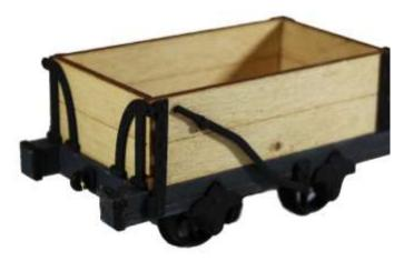
A choice of couplings is included in this kit. You can either assemble the wagon with side "dumb buffers" and a central hook for a 3 link chain (see above) or if you prefer a centre buffer (for greater compatibility with the rest of your stock), a pair of Penrhyn style wagon buffers are also included (see right).
