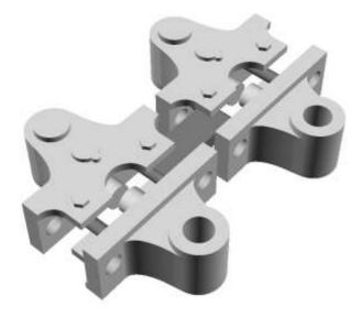
Clean out any printing dust in the axle holes by "twizzling" a 3mm drill bit in them
